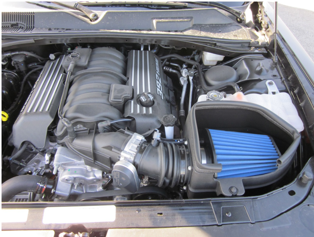
o) This is how your MOPAR air intake system should look when properly installed.
