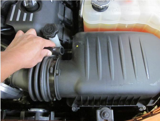
c) Detach the valve cover breather hose from the air box.
