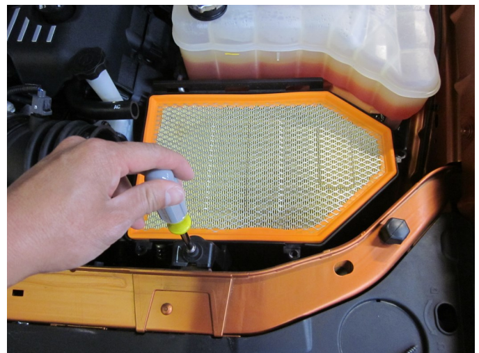
f) Loosen and remove the M6 air box mounting bolt. This bolt will be reused in step 3j).
