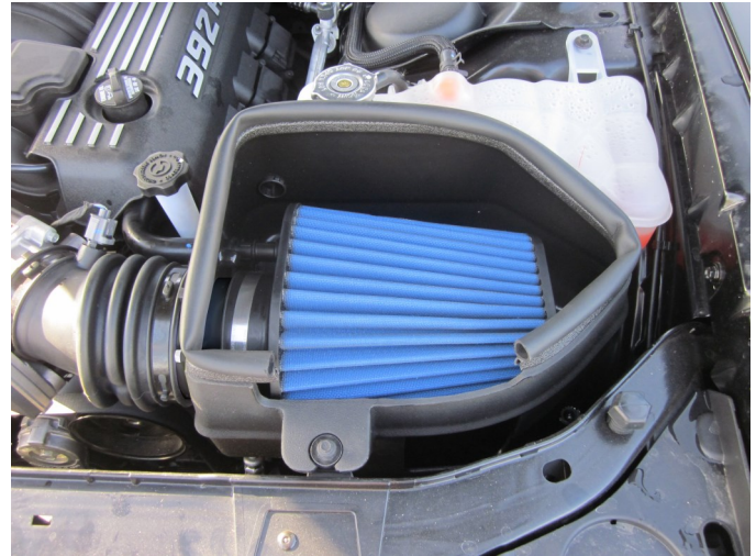
n) Edge trim installed.
