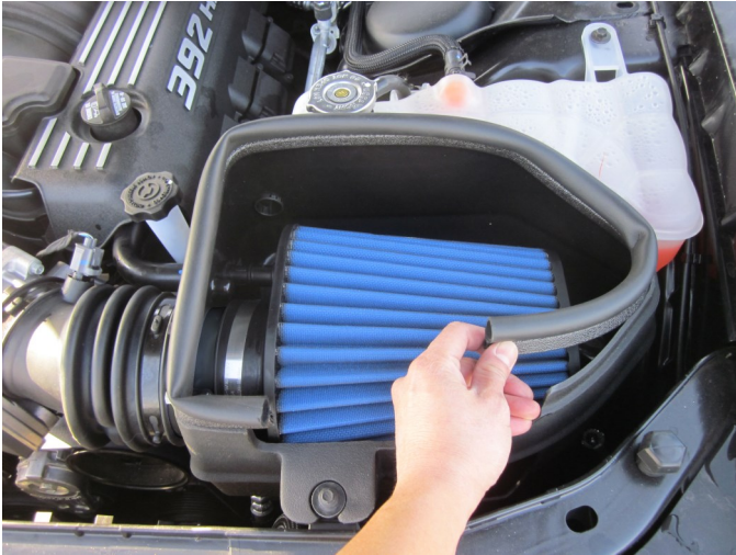
m) Attach the supplied rubber edge trim to the top of the air box.
