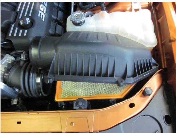
e) With the M6 screws removed, un-hinge and remove the air box lid from the air intake hose.
