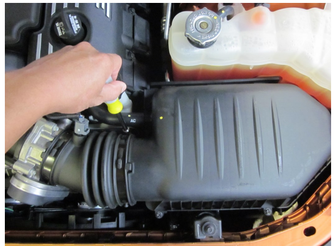
b) Loosen the hose clamp securing the air inlet tube to the air box.
