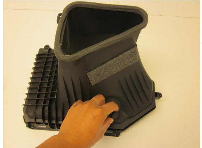
h) Remove the rubber bushing from the air box base. This will be transferred to the MOPAR air box in step 3b).
