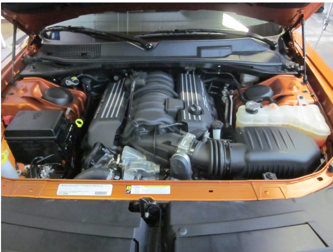
a) Your stock air intake system should look like this.
